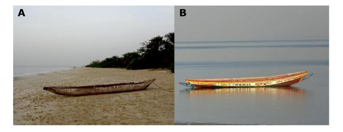
The two predominantly used vessels in the small-scale fishery within the Bijagós Archipelago, the dug-out canoe (A; approximately 5 to 8 meters in length) and the larger pirogue (B; ~15 meters in length). Whereas the dug-out canoes are mostly solely human-powered, the pirogues are mostly used by one or multiple outboard engines.
